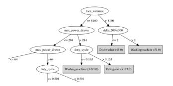
At left is an example decision tree output. Based on features in the data (which we calculate using the 1-second power readings), the algorithm first trains on seen data, meaning data that is labeled as "Washing\_Machine," and then attempts to test on unseen data, meaning data that is not labeled but still has the features. We hope to identify correctly given those features. I spent a good portion of my time
